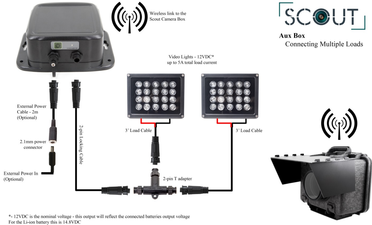
Figure 1 – Scout Aux Box Connections
